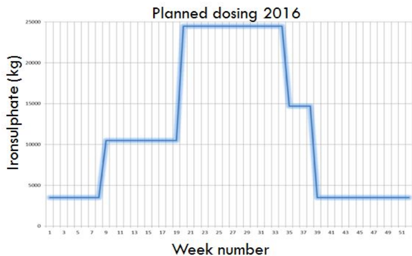
Figure 6: Planned dosing of Iron sulphate (kg) in the different weeks of 2016. The amount ranges from less than 5000 kg in winter to 25000 kg in the summer. In the summer there is more biological activity due to a higher average temperature of the water, resulting in a more pressing need to remove the phosphate from the river water to prevent (blue) algae blooms.
